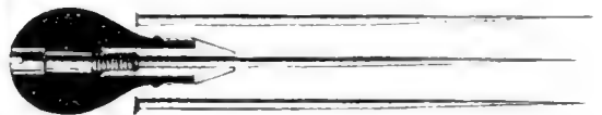
The Ice Pick Illustrated Below Is Made of Separable Parts. The Handle Is Provided with Jaws Which Clamp Tightly or Release the Three Removable Picks
